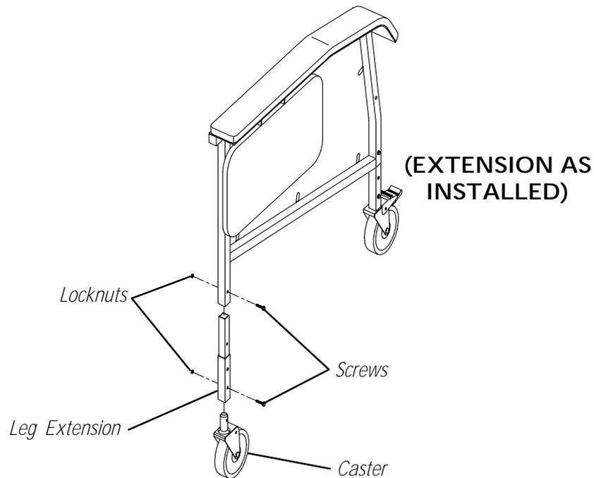
**FIGURE 1 - INSTALLING 5-INCH LEG EXTENSION KIT - MODEL 6908A**
