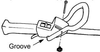
**NOTE:** Knob must be assembled on the right hand side of the unit as shown in the illustration.
