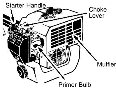
6. Pull starter rope handle sharply until engine sounds as if it is trying to start, but do not pull rope more than 6 times.
