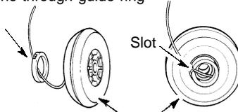
3. Rest guide ring on spool and place line through slot. Allow line to extend 4 - 6 inches (10 - 15 cm) from center of spool.
