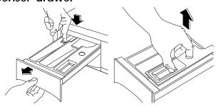
the drawer from the machine, press the button in the rear left-hand corner.
