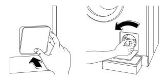
Place a container under the filter and unscrew it; some water will come out of the filter.
