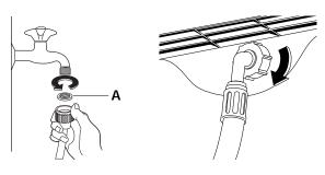
Connect the water inlet hoses to separate taps for cold and hot water with a 3/4" thread after having inserted the small filters "A" supplied with the machine.
