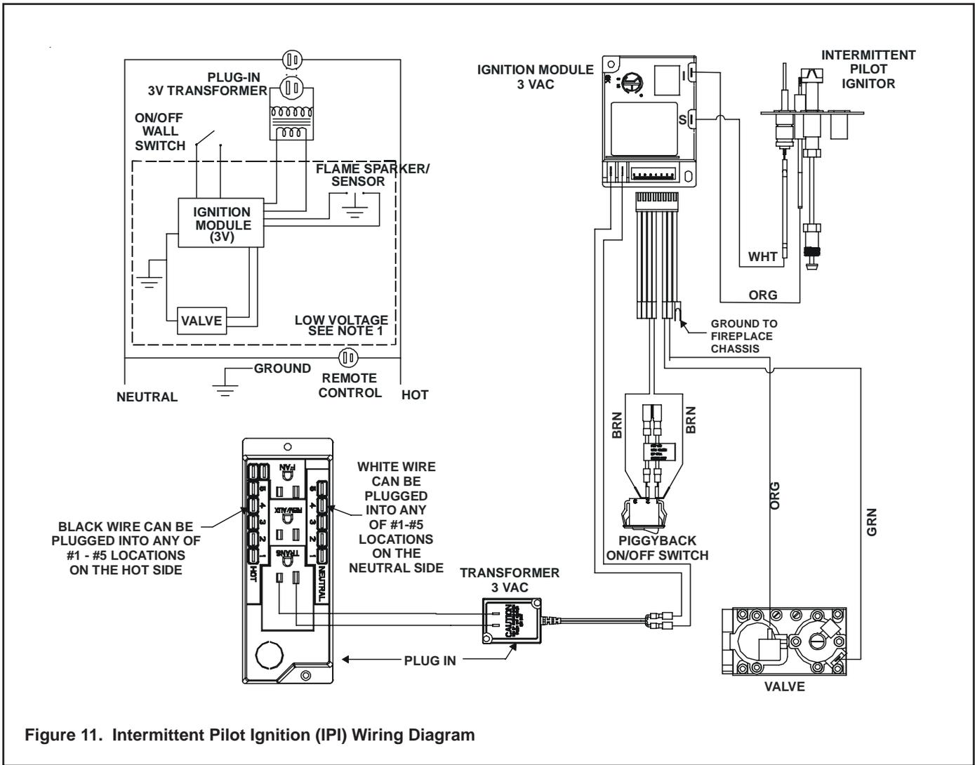
Figure 11. Intermittent Pilot Ignition (IPI) Wiring Diagram
