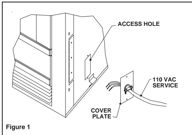
2. Feed the electrical service wires through the Romex clamp and secure the wires to the clamp.
