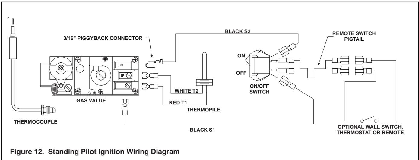
Figure 12. Standing Pilot Ignition Wiring Diagram
