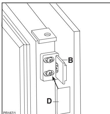
If the appliance is fixed to the side of the kitchen unit, simply slacken the screws in the fixing brackets (D), move the brackets as shown in the figure and re-tighten the screws. Then fit cover (E).
