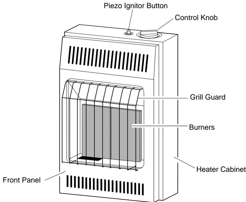
Figure 1 - Model VN10TA Vent-Free Natural Gas Heater
