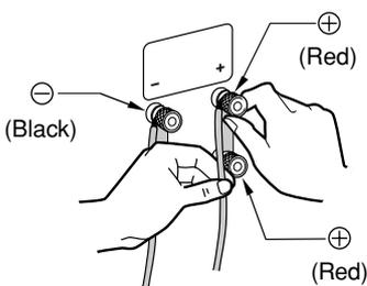
Rotate the speaker terminal knob counterclockwise and fit the speaker cord into the groove. Then rotate the knob clockwise to secure the cord.
