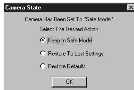
In a system having the PI-MAX camera, this dialog box appears when the software is booted. It allows the user to set the camera start-up state. The three selections are:
