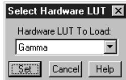
The Hardware LUT dialog box (Figure 243) is opened by clicking on Hardware LUT on the Acquisition menu. Its purpose is to determine how video will be mapped to a video monitor display. The selection doesn't affect the data in any way, but rather only in the way it is displayed on a video monitor. A brief description of the available selections follows.
