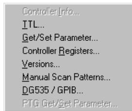
The Diagnostics menu, which is accessed by selecting Diagnostics on the Setup menu, allows access to a number of diagnostics functions. *Some of the listed diagnostics functions are primarily intended for factory hardware development.*
