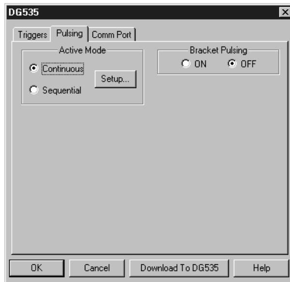
Selects the Continuous or Sequential Pulsing mode and allows access to the setup screens for Continuous or Sequential Pulsing. Allows bracket pulsing of the PI-MAX MCP to be switched ON or OFF. *See Chapter 13 for additional information on controlling a pulser/timing generator.*
