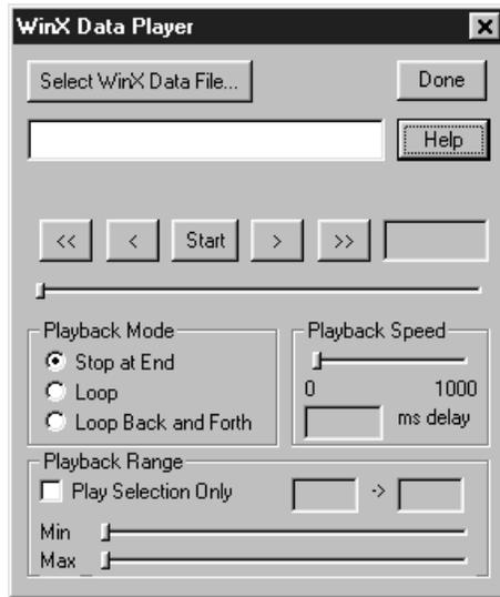
The WinX32 Data Playback Snap-In plays back as a movie a multiple-frame image file collected with the WinX32 program. The “movie” is displayed in the standard Data Window.
