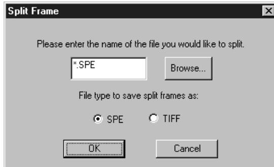
Allows you to split a multi-frame file into its constituent frames. The original file is retained and each frame is saved in a separate located in the same folder as the original. Numbers are appended to indicate the frame number. For example, if the original file contained ten frames and was named **Minney.spe**, the individual frame files would be named **Minney1.spe**, **Minney2.spe**... **Minney10.spe**.
