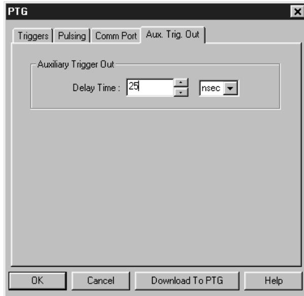
Sets the delay to the Auxiliary Trigger Output with respect to the PTG trigger time. The minimum delay is 25 ns and the longest is 10 ms. The resolution is 0.04 ns.
