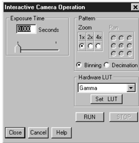
This box is opened by clicking on **Video Focus** from the Acquisition menu (PentaMAX Controller). This dialog box allows focusing to be quickly accomplished in “real time” by making the adjustments while observing the image on a video monitor connected to the controller’s video output as described in the PentaMAX manual. Note that data collection doesn’t take place and the image will not appear at the computer monitor as long as the interactive dialog box is open.
