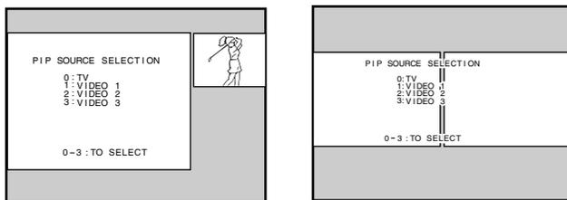
While the above menu is on the screen, you can select the desired signal input source by pressing the corresponding number button (0-3).
