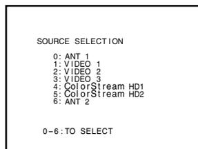
Pressing TV/VIDEO on the remote control displays the current signal source (press TV/VIDEO again or 0-6 to change)
