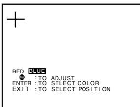
9. Press ▲▼◀▶ to converge the red or blue line into the green line, which will turn completely white when correctly adjusted. Repeat steps 8 and 9 until you see two single crossed white lines.
