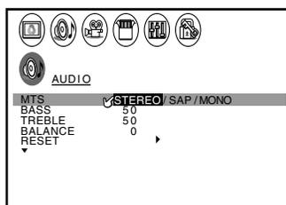
You can leave your TV in STEREO mode because it will automatically output the type of sound being broadcast (stereo or monaural). The word “STEREO” or “SAP” displays in yellow in the menu when the TV receives the signal.
