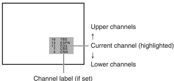
2. Repeatedly press or hold Channel ▲ or ▼ while the SpeedSurf mode is on-screen to scroll the channel list. Release the button to display the highlighted channel.
