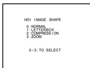
While the above menu is on-screen, select the desired picture size by pressing the corresponding number button (0–3).
