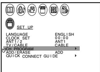
5. Press ◀ or ▶ to start channel programming. The TV will automatically cycle through all the TV or Cable channels (depending on which you selected), and store all active channels in the channel memory.
