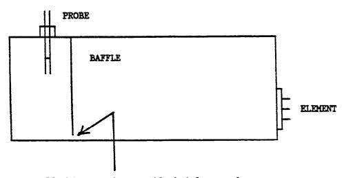
If this area becomes blocked from scale buildup, false water levels can be sensed by the electrodes. The generator must be delimed and cleaned. This is a fairly frequent cause of element failure.
