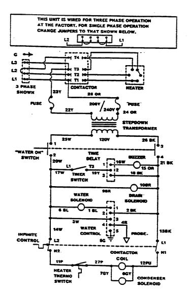
SINGLE PROBE UNIT 7/29/79 thru 8/1/82 DO NOT ATTEMPT ANY MAINTENANCE UNLESS THE ELECTRIC SUPPLY HAS BEEN COMPLETELY DISCONNECTED. IF A DISCONNECT SWITCH HAS NOT BEEN PROVIDED, REMOVE ALL FUSES FROM THE CIRCUIT AND LOCK THE FUSE PANEL SO THAT THE FUSES CANNOT BE ACCIDENTALLY REPLACED.
