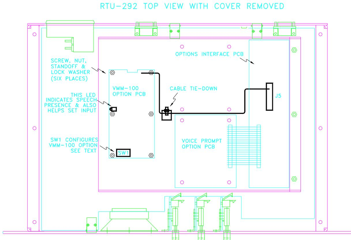
**Figure 7-3 VMM-100 Option Installation**
