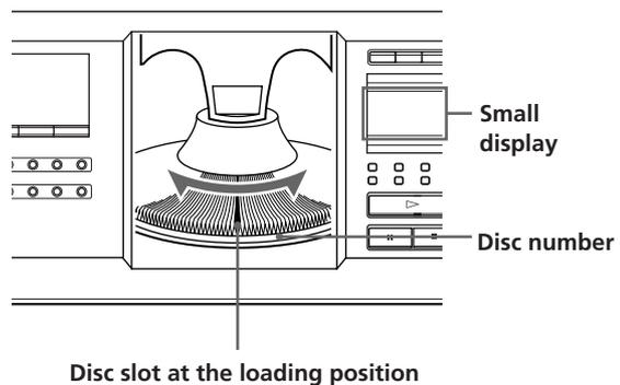
Disc slot at the loading position
