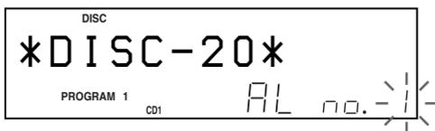
**3** To program a whole disc, skip this step and go to step 7. To program a whole album or an MP3 file, go to step 4. To program an audio track, turn the AMS dial until the desired track number appears in the display and go to step 7.
