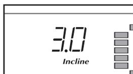
and the incline level of the treadmill. Note: Each time the incline changes, the display will show the incline setting.
