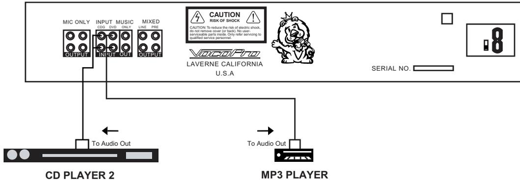
While both input channels are designated with a device name (DVD and CDG), any compatible device can be connected to them. *NOTE: If there is a needed video connection from one of the source players, connect the video straight from the source player to the TV or display device. The device names are for convenience only, and not meant to prevent one from connecting a different compatible device.*
