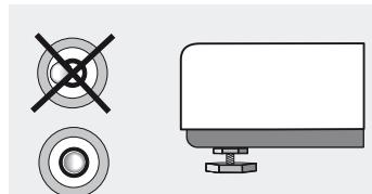
Set up the weighing platform at the place required. Use the water level and the adjustable feet to ensure that the scale is positioned horizontally.
