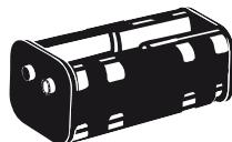
At the bottom of the scale you can find the battery holder. 8 batteries "baby cells 1,5 C" or NiCd-accumulators of the same size are required. The lenght of operation depends on the quality of the batteries or accumulators, e.g. at an accucapacity of 1,4 Ah appr. 8–10 operation hours. During accu resp. battery operation the background light of the display is switched off automatically.
