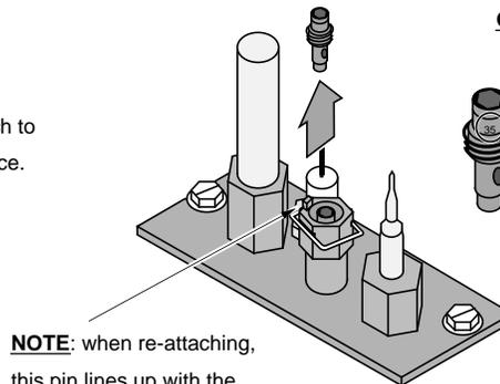
**NOTE:** when re-attaching, this pin lines up with the notch in the pilot hood.
