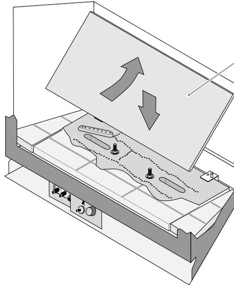
**NOTE:** The rear fireback must be installed as shown below for the brick pattern to line up with the side firebacks.
