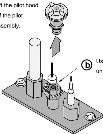
**b** Use a hex wrench to unscrew the orifice.
