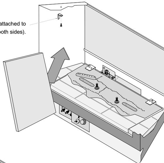
Replace the clip to secure the side fireback (both sides).
