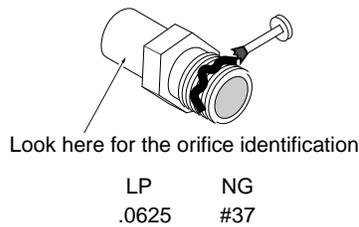
**d** Screw the LP orifice in so the orifice shoulder protrudes 5/16" (indicating full insertion).
