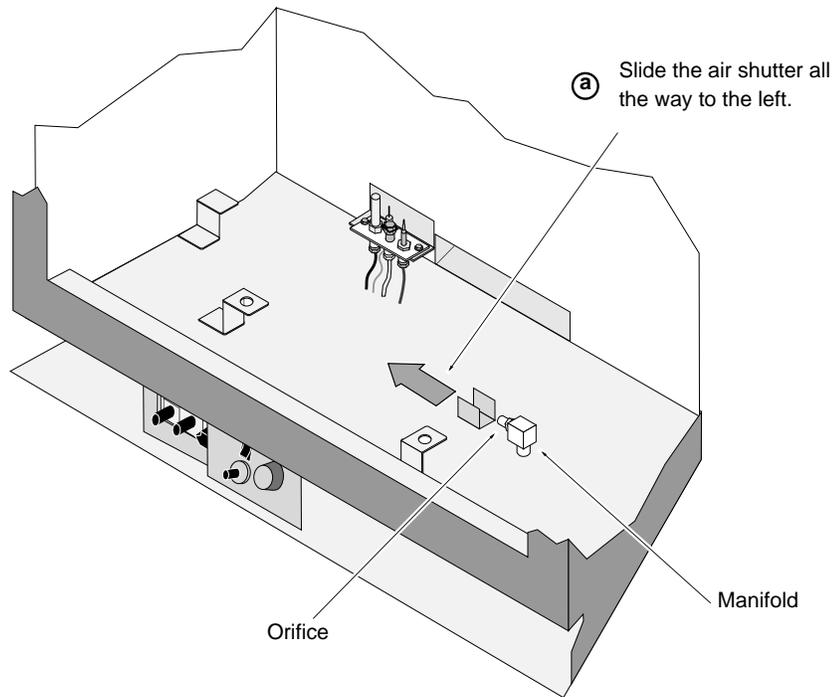
**b** Use a 1/2" open end wrench to unscrew the orifice.
