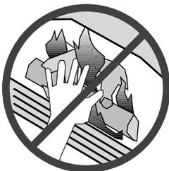
Do not place anything inside the firebox (except the included fiber logs). If the fiber logs become damaged, replace with Travis Industries log set.
