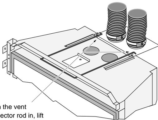
Push the vent connector rod in, lift slightly, and line it up so the tabs on the end of the rod engage the hooks on the vent connector
