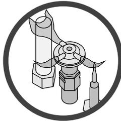
The pilot flame must contact the thermopile and thermocouple (see the illustration to the left). If it does not, turn the gas control valve to "OFF" and call your dealer.
