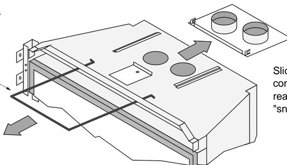
Slide the connector to the rear. It will "snap" out.
