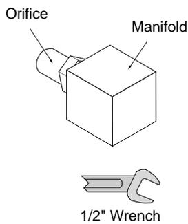
**c** Apply thread sealant to the LP orifices prior to installation. Use the chart below to identify the correct orifices.
