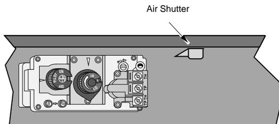
**NOTE:** The logs must be installed correctly to monitor the flame while adjusting the air shutter.
