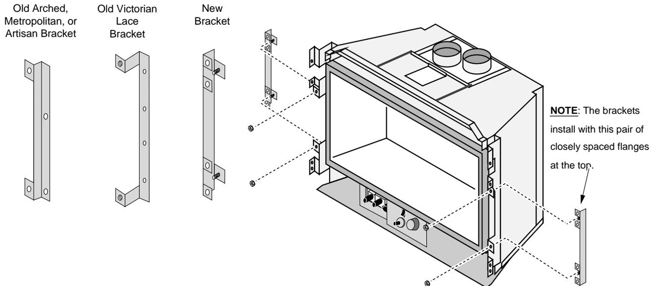
Install the face mounting brackets to the heater with the included nuts.
