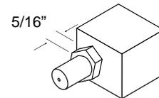
4 Remove the pilot orifice following the instructions below. Replace with the propane pilot orifice
