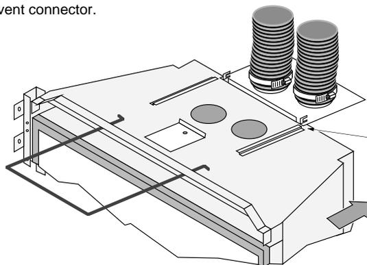
Slide the insert into place, lining up these guides with the edges of the vent connector.
