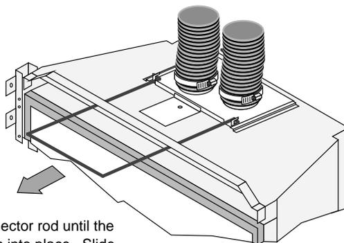
Pull on the vent connector rod until the vent connector snaps into place. Slide the vent connector rod in to conceal it.
