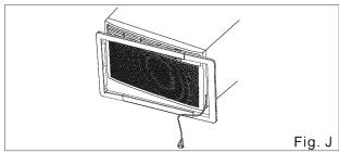
**NOTE:** Be sure to route the cord through the trim frame before placing the trim frame on the unit.
