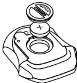
FIGURE 13: BATTERY INSTALLATION
