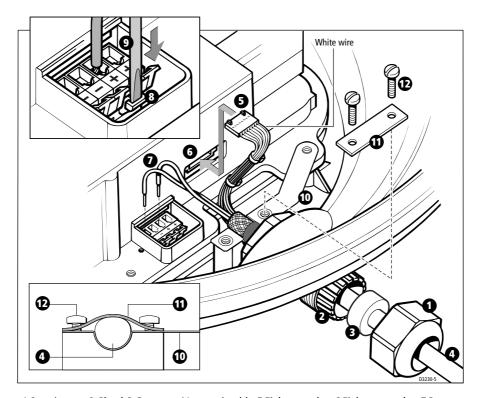
1 Securing nut 2 Gland 3 Grommet 4 Inter-unit cable 5 Eight-way plug 6 Eight-way socket 7 Power cores (2 or 4) 8 Terminal clamp 9 Screwdriver 10 Earthing clamp 11 Top clamp 12 Clamp screws
