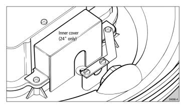
4. Remove the drain tube from inside the base of the scanner, and insert it into the drain hole as shown in the following diagram. Pull the tube gently from outside the scanner so that it clips into place.
