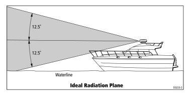
Planing hull vessels, and some displacement hull vessels, adopt a higher bow angle when the vessel is at its cruising speed. In many cases this substantially alters and raises the radar's main radiation plane, and can cause poor detection of nearby targets. It may be helpful to lower the radar beam back towards the parallel, by shimming the rear of the radar, so that the beam points slightly downwards with respect to the waterline when the vessel is at rest.
