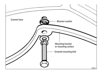
You may need to use longer M8 mounting bolts to secure the scanner if you have used shims to lower the radar beam.
