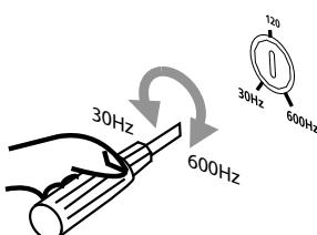
**(Eng)** The cut frequency is selectable between 30 to 600 Hz.
