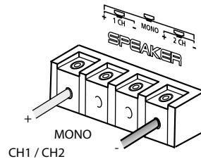
**(Eng)** Minimal acceptable Impedance 2 ohm. To adhere itself to the illustrations for the connections.
