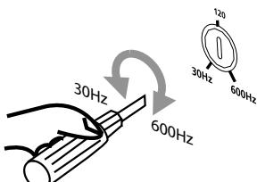
**(Eng)** The cut frequency is selectable between 30 to 600 Hz.
