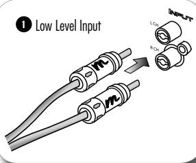
**(Eng)** Connect the output Audio coming from the car radio, in to the Low level input of the amplifier.
