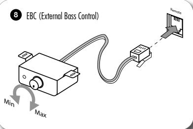
**(Eng)** Through control Remote EBC, it is possible to control the level of the Volume of the amplifier. Placed control EBC in the front part of the vehicle.
