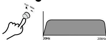
**(Eng)** The cut frequency is selectable between 30 to 600 Hz.
