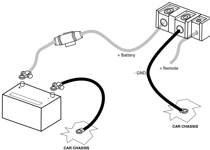
**(Eng)** Connect the Positive (+12V) directly to the Battery of the car. To make sure itself to insert a fuse of adequate amperage in order protect the system. Connect the Ground in to the car chassis, close as possible to the amplifier.
