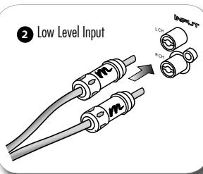
**(Eng)** Connect the output Audio coming from the car radio, in to the Low level input of the amplifier.
