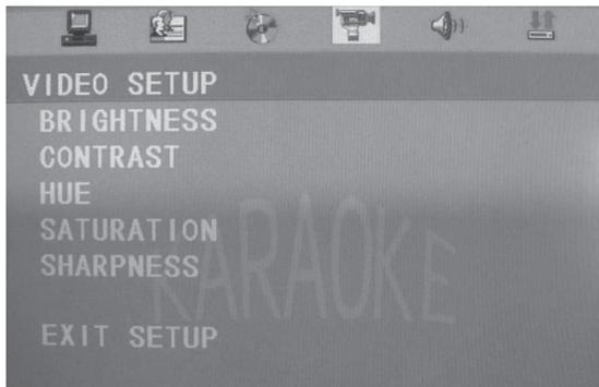
Unload the disc, press SETUP KEY to open the Setup MENU, then press Direction KEY [◀/▶] to select VIDEO SETUP (see image above). The SUB-MENU contains:
