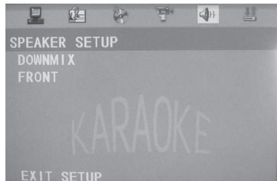
Unload disc, press SETUP KEY to open the SETUP MENU, then press Direction KEY [◀/▶] to select SPEAKER SETUP. The SUB-MENU contains:
