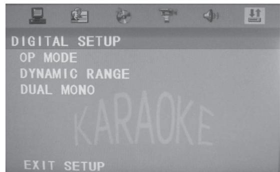
Unload the disc, press SETUP KEY to open SETUP MENU, then press Direction KEY [◀/▶] to select DIGITAL SETUP. The SUB-MENU contains:
