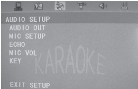
Unload the disc, press SETUP KEY to open the SETUP MENU, then press Direction KEY [◀/▶] to select the AUDIO SETUP. The SUB-MENU contains:
