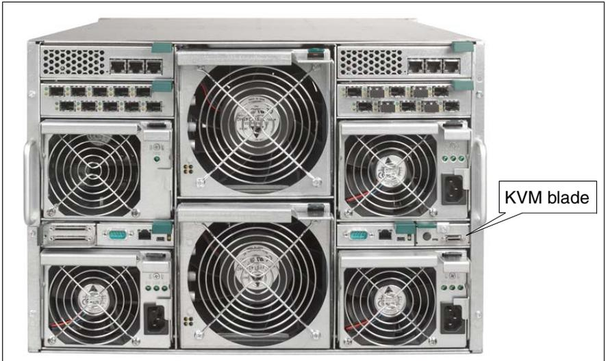
Figure 84: Position of the KVM blade
