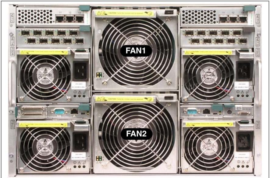
Figure 95: PRIMERGY BX600 S2 basic unit: fan units
