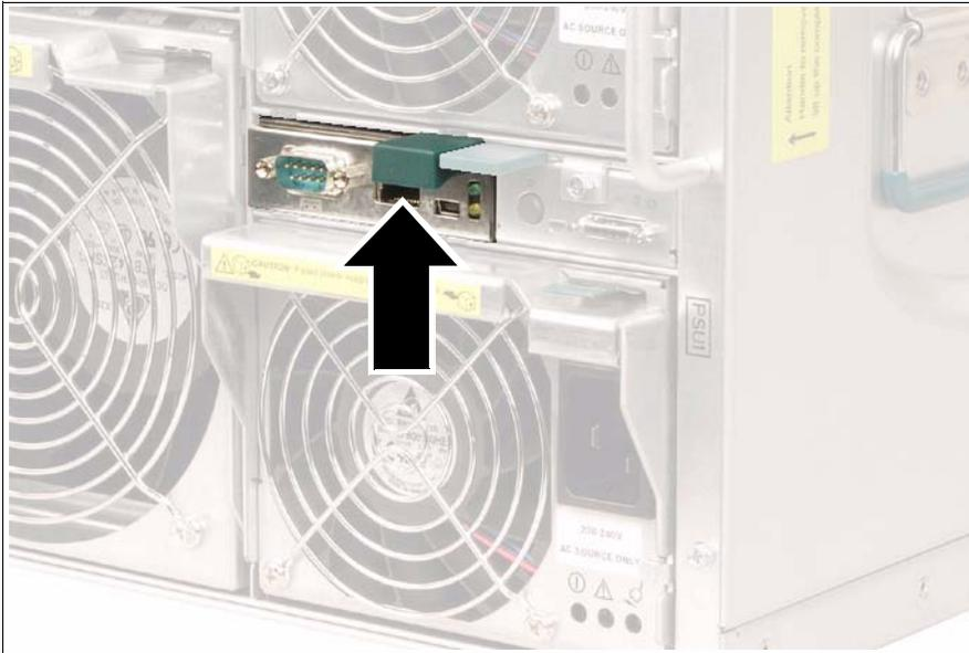
Figure 81: Disengaging the management blade
