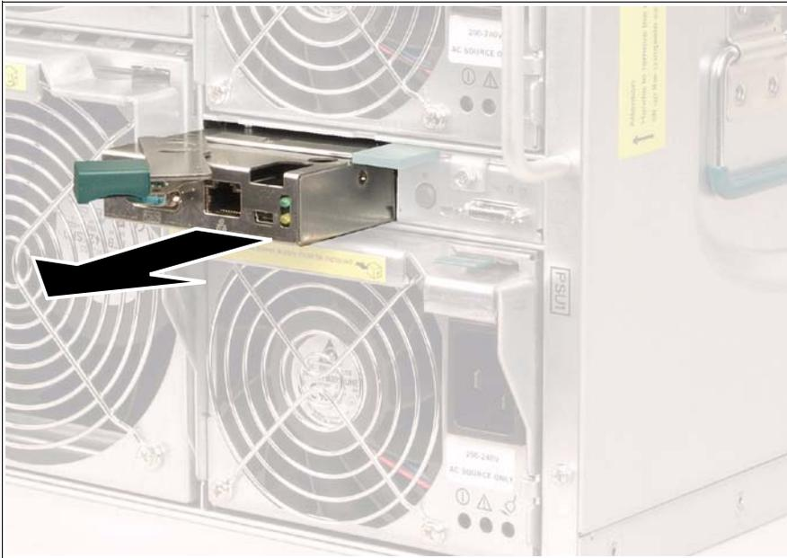
Figure 83: Removing the management blade
