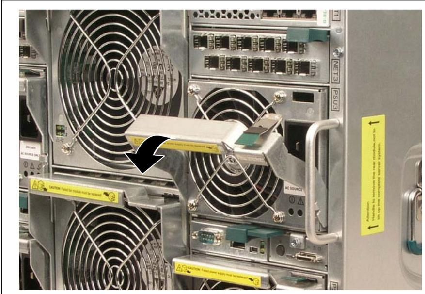
Figure 92: Removing the power supply unit
