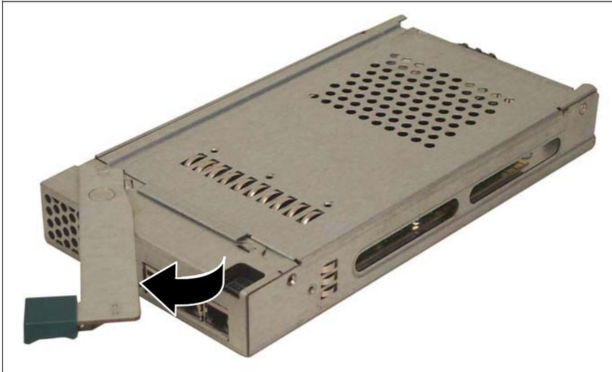
Figure 50: Disengaging the switch blade
