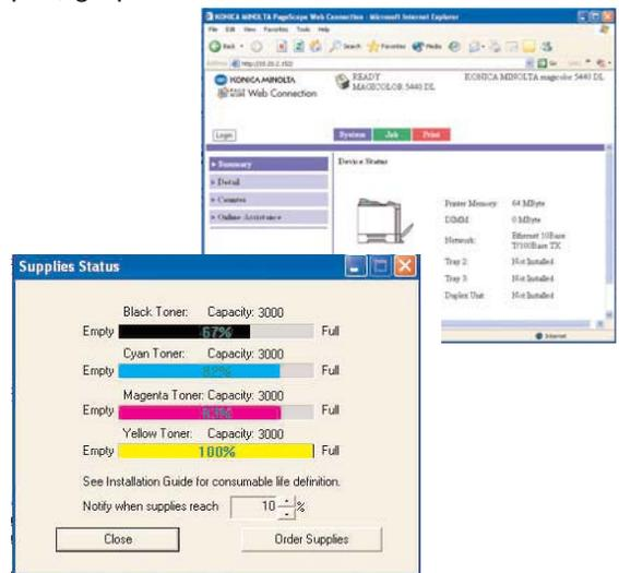
PageScope Web Connection and the Status Monitor provide easy methods for checking print job and supply status.
