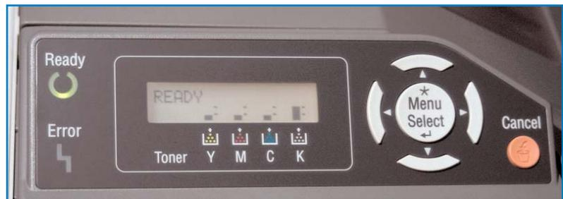
From the front keypad, users can access the menu system to print a Configuration Page. This sheet details information on all supplies as well as showing the number of pages printed, options installed, network setup, and engine settings.
