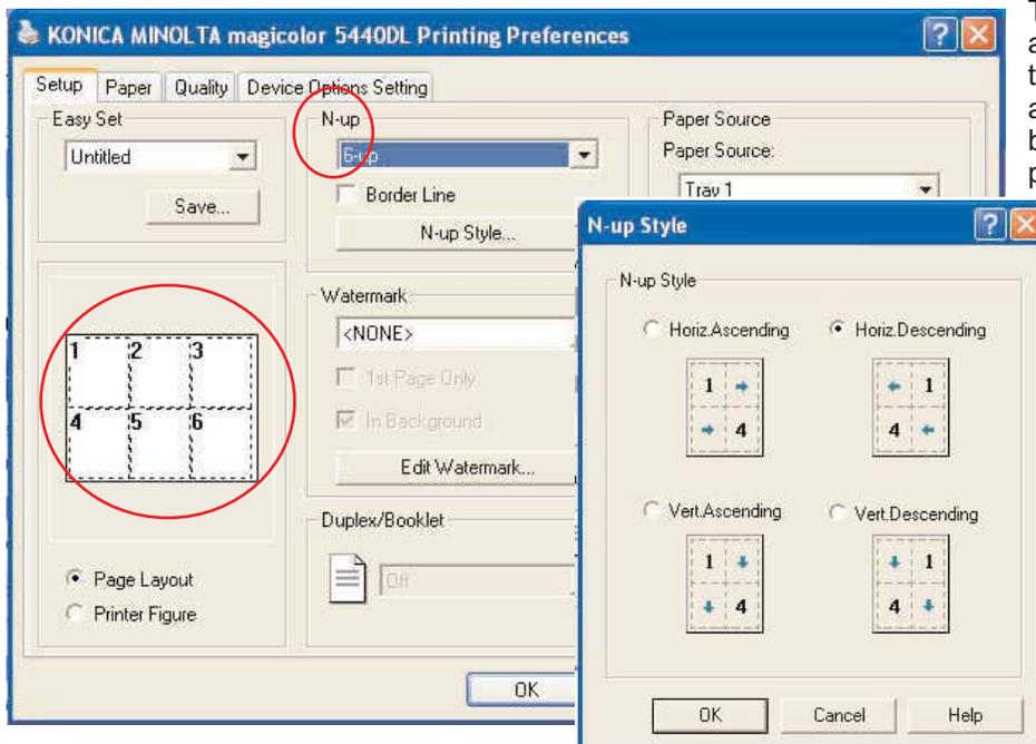
The magicolor 5440 DL driver also has an N-up option that allows users to print their multi-page documents with 2, 4, 6, 9 and 16 pages on a single sheet. Add a border line and select the flow of the pages across the sheet using easy to understand driver settings.
