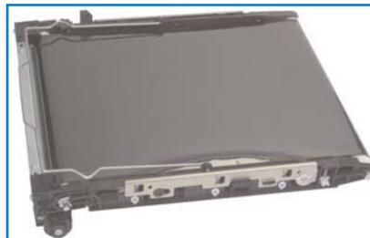
The magicolor 5440 DL also has a transfer belt that takes the image composed of toner and transfers it to the print media as the media passes through the engine.
