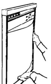
**5.** Push in on door panel(s) near the top and slide panel(s) and spacer up inside bottom of control console.
