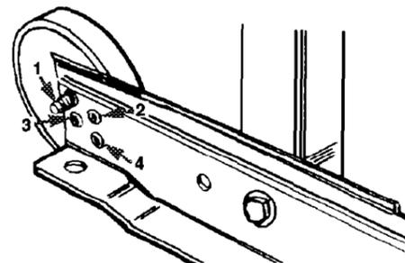
**6.** The dishwasher is shipped to be installed in cabinet opening with a 34" height. Measure height of cabinet opening from the front edge of the underside of cabinet opening to floor. Check chart for that height opening. Put the wheels in the required position. The dishwasher should be installed as level as possible from front to back. Loosen and then turn front levelers the number of times indicated in the chart.
