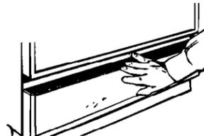
**4.** Line up edges of top trim with sides of access panel frame. Tilt back of trim down and slide into place. Snap front of trim down to cover top edge of access panel.
