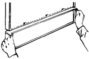
**2.** Carefully slide color access panel upwards and remove. Do Not remove spacer.
