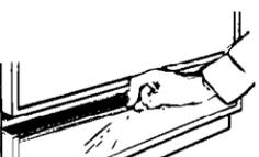
**13.** Insert wood access panel into access panel frame. Slide panel down into groove along bottom of access panel frame. It may be necessary to remove top mounting screws and tilt access panel forward to install some wood panels.
