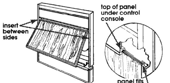
**5.** Insert top of wood door panel between sides of door frame about 3" below console. Rotate wood door panel down against dishwasher door. Slide top edge of wood door panel under bottom edge of console. Press lower portion of wood door panel in place between sides of door frame.
