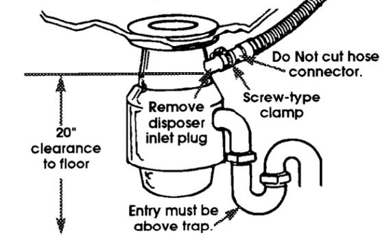
If local plumbing codes permit, dishwasher drain hose may be connected directly to disposer. Most disposers have 7/8" connectors or special connectors are available at plumbing supply houses. **Be sure to remove the disposer plug before connecting the drain hose.**
