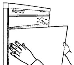
**4.** Bow door panel(s) and insert other side of door panel(s) into door frame.
