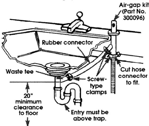
Drain hose to air gap to disposer.
