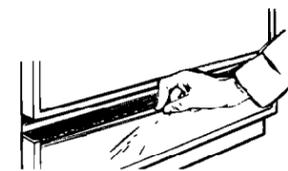
**3.** With desired color facing out, bow access panel and insert into access panel frame. Slide panel down into groove along bottom of access panel frame.
