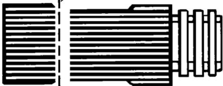
If connecting drain hose to an air gap or waste tee, cut end of drain hose as shown.
