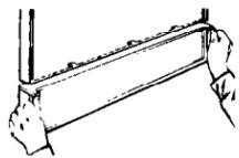
**12.** Carefully slide color access panel and spacer upwards and remove. Save color access panel and spacer for future use.
