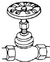
**3.** Flush water line into a bucket to get rid of any particles that may clog inlet valve. Turn shutoff valve to the "OFF" position.
