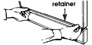
**2.** Slide panel(s) down to clear console. Use both hands to bow top and bottom edge of door panel(s). Remove panel(s) from door. **Do Not remove spacer.**
