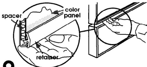
**9. Important:** Run fingers along bottom of retainer to check that retainer is lower than the lower door frame.
