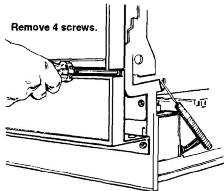
**5.** Remove the 4 screws attaching access panel and toe panel to dishwasher using a 1/4" hex socket, nut driver or Phillips screwdriver. Remove access panel and toe panel.
