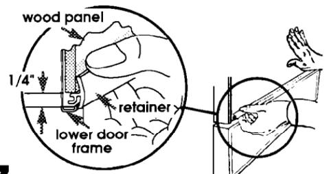
**7.** Insert retainer over lower edge of door frame while holding wood door panel up.
