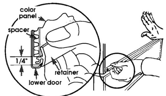
**7.** Insert retainer over lower edge of door frame while holding door panel(s) and spacer up.
