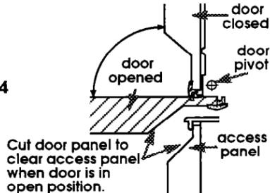
Cut door panel to clear access panel when door is in open position.
