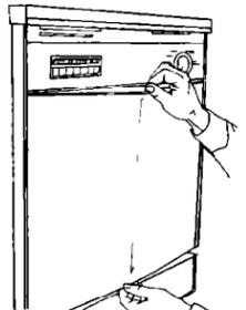
**3.** With desired color facing out, insert one side of door panel(s) into one side of door frame.
