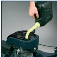
2. Fill the tank to approximately 2.5 cm below the lowest portion of the neck to allow for fuel expansion.
