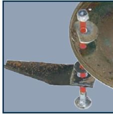
**Note.** Use a wooden block to stop the blade from turning. The 4 blades should be tightened fully but check to ensure they can still swing back if they were to hit a solid object.
