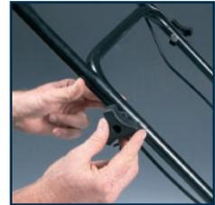
4. Position the handle bar over the lower handle and insert the two locking knobs. Tighten to secure the handles together and in place.
