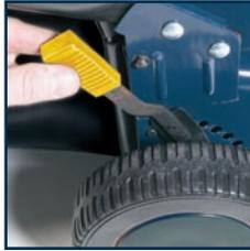
**Note.** If you are unsure of which cutting height to use, begin with a high setting and trial a small section of lawn, then check the appearance of the lawn. Then readjust if necessary
