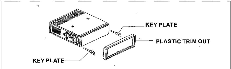
If you want to take CHASSIS out of the SLIDE BRACKET HOUSING, first remove the PLASTIC TRIM OUT of the both sides away, then insert the two KEY PLATE into left and right side of chassis as above illustration.
