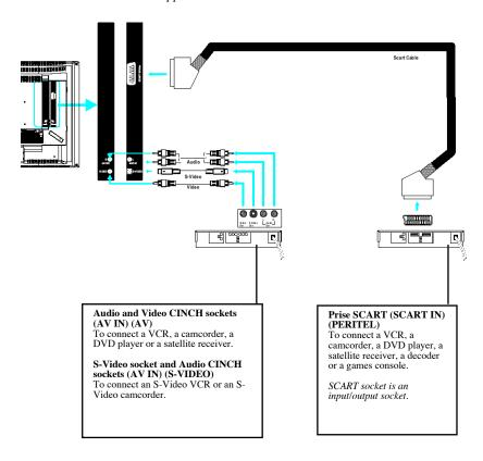
To display images from the connected appliance, select the input source by pressing the AV button on the remote control.
