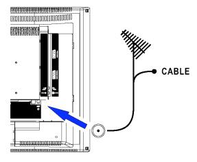
The aerial socket (75 Ohms - VHF / UHF / cable) can be used for connecting an external aerial or other equipment fitted with a modulator (video recorder, satellite receiver, etc.).
