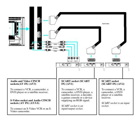
To display images from the connected appliance, select the input source by pressing the AV button on the remote control.
