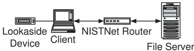
**Figure 4.** Experimental Setup
