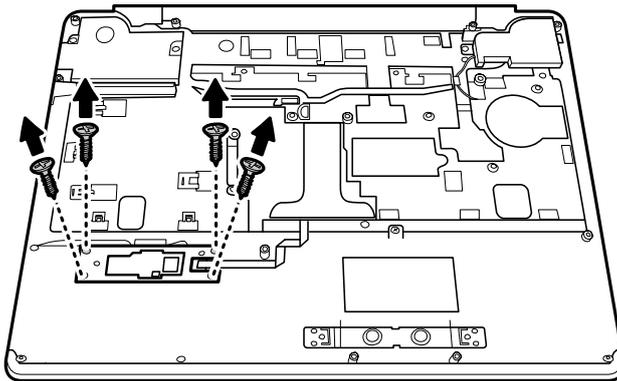
Figure 4-49 Removing the fingerprint module bracket screws
