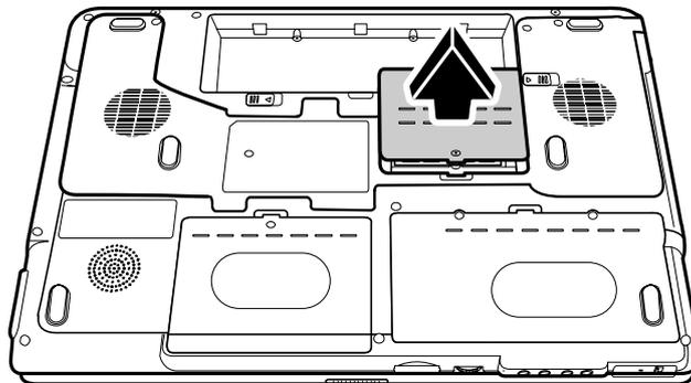
Figure 4-17 Removing the expansion memory module cover
