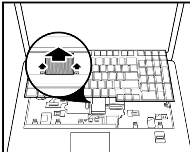
Figure 4-29 Disconnecting the keyboard cable
