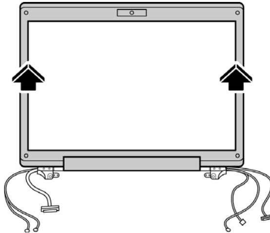
Figure 4-75 Removing the display mask screws
