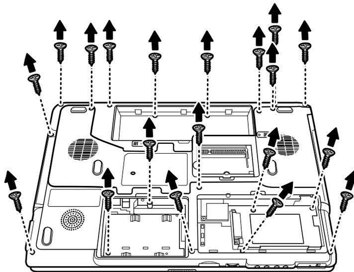
Figure 4-42 Removing the top cover (back panel screws)
