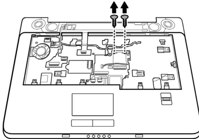
Figure 4-38 Removing the wireless LAN unit screws
