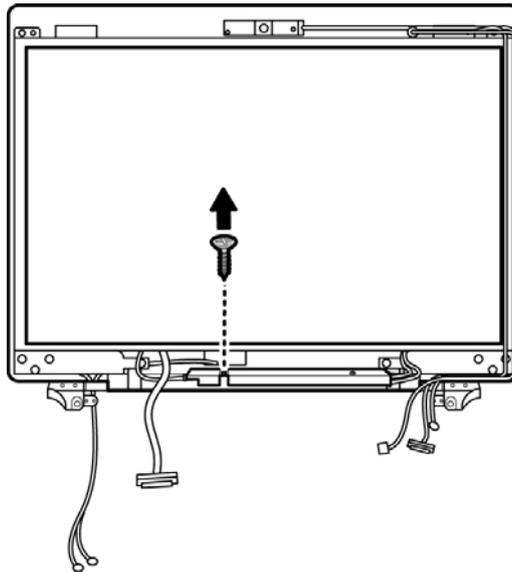
Figure 4-76 Removing the FL inverter board screws
