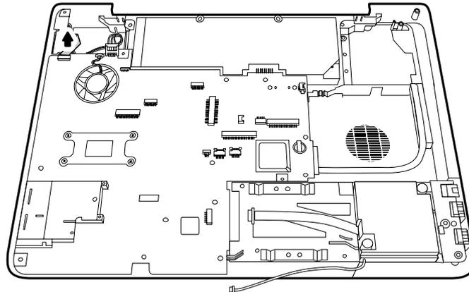
Figure 4-62 Removing the VGA PCB FFC cable
