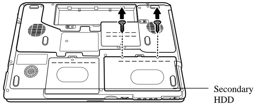
Figure 4-13 Releasing the secondary HDD door screw
