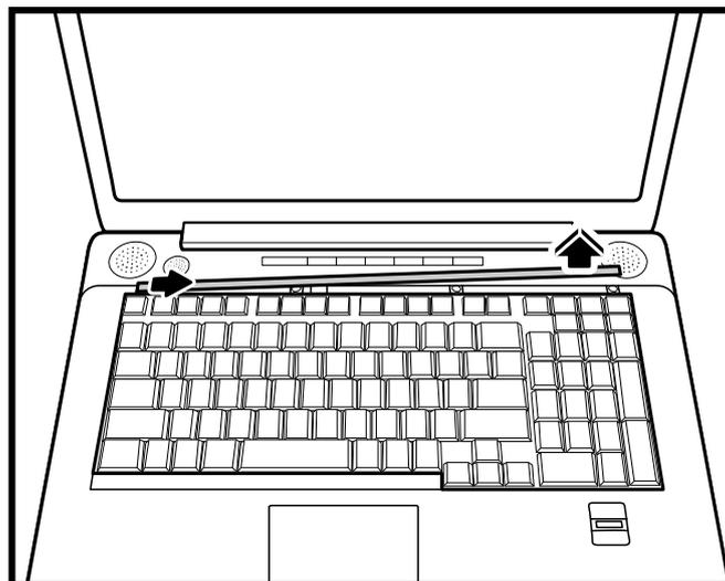
Figure 4-27 Removing the keyboard cover
