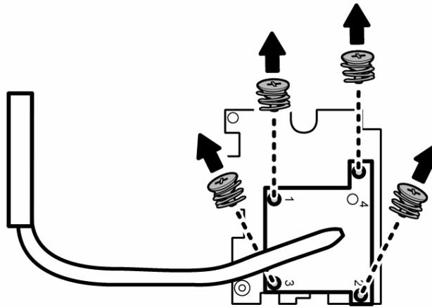
Figure 4-67 Removing the VGA heat sink
