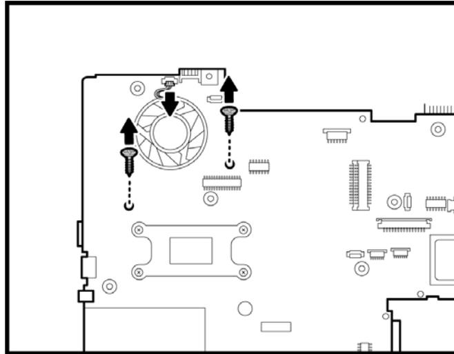
Figure 4-70 Removing the fan connector and screws
