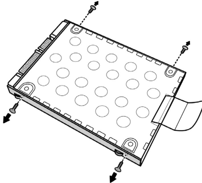
*Figure 4-12 Removing the HDD screws from brackets*
