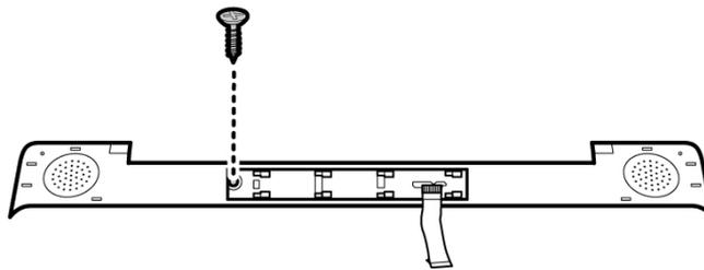
Figure 4-35 Removing the function button board screw
