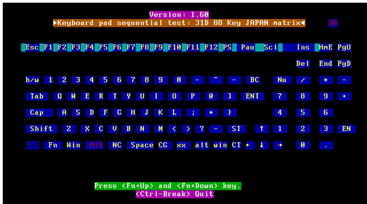
**NOTE:** The “Fn” key cannot be tested in the keyboard test. To determine whether the “Fn” key is working correctly, press “Fn+F6 ” or “Fn+F7 ” keys to check if LCD display brightness change gradually.
