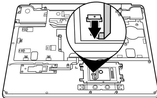
Figure 4-47 Disconnecting the touch pad FFC cable
