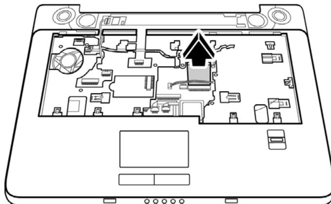
Figure 4-39 Removing the wireless LAN card
