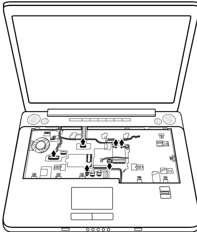
Figure 4-30 Disconnecting cables
