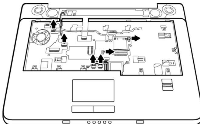
*Figure 4-43 Removing the cables*
