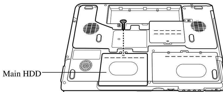
Figure 4-9 Releasing the main HDD door screw
