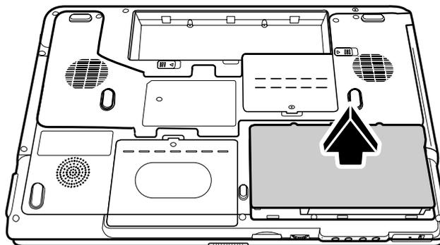
Figure 4-14 Removing the secondary HDD door
