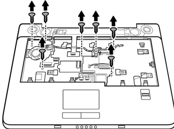
*Figure 4-44 Removing the top cover (front panel screws)*
