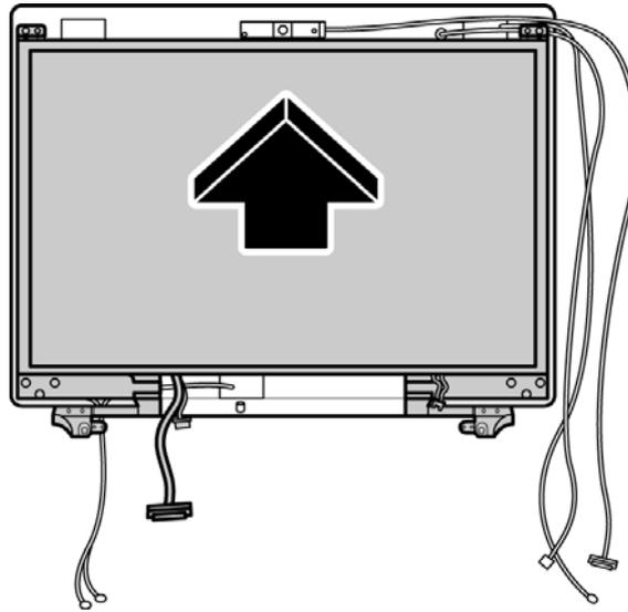
Figure 4-80 Removing the LCD Module
