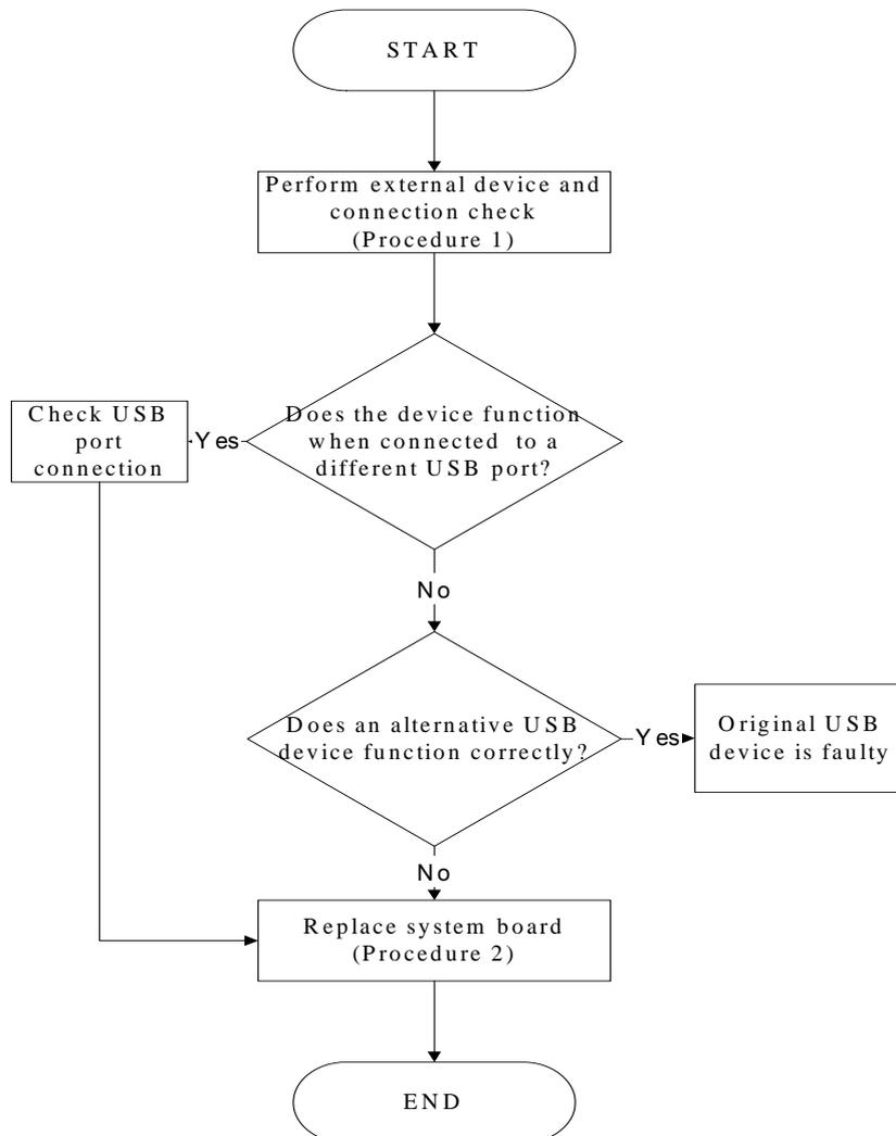
Figure 2-5 External USB device troubleshooting process
