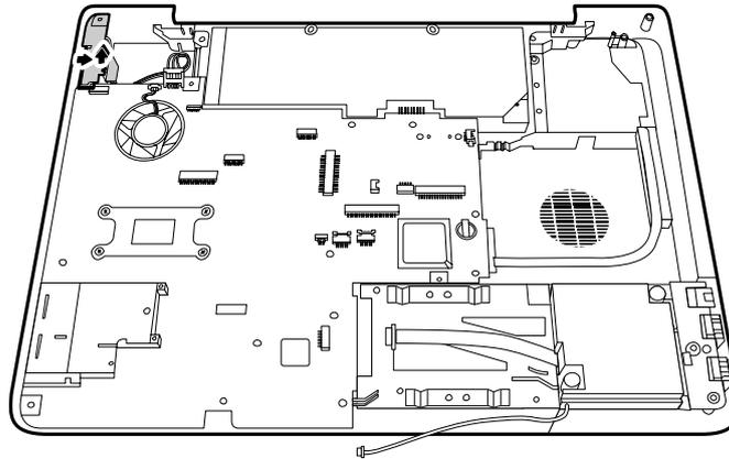
*Figure 4-64 Removing the VGA PCB*
