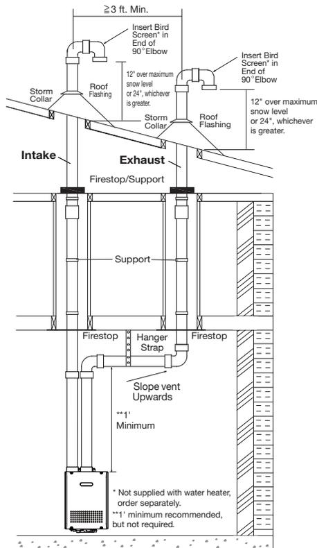
When choosing intake and exhaust terminations, you must use the same type of elbow (i.e. both 45° elbows, or both 90° elbows). This will help with proper combustion by putting both terminations in the same pressure zone.
