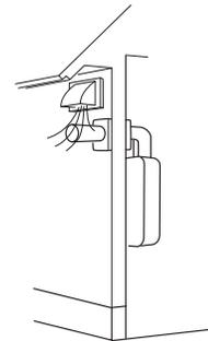
State of California: The water heater must be braced, anchored or strapped to avoid moving during an earthquake. Contact local utilities for code requirements in your area or call: Electrolux Home Products, Inc. at 1-888-360-8557 and request instructions.
