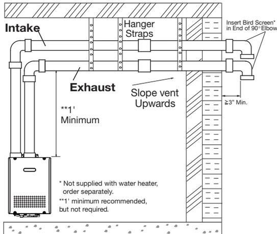
When choosing intake and exhaust terminations, you must use the same type of elbow (i.e. both 45° elbows, or both 90° elbows). This will help with proper combustion by putting both terminations in the same pressure zone.
