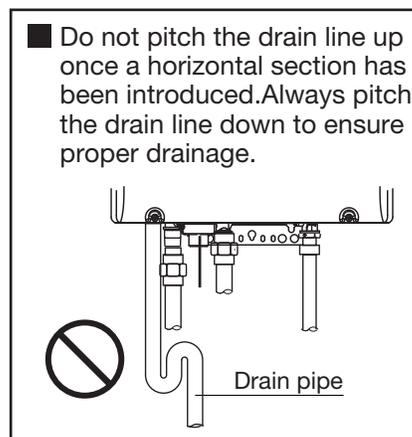
Condensate piping to floor drain
