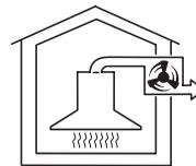
The EXT models are designed to be connected to an external motor located outside the room.
