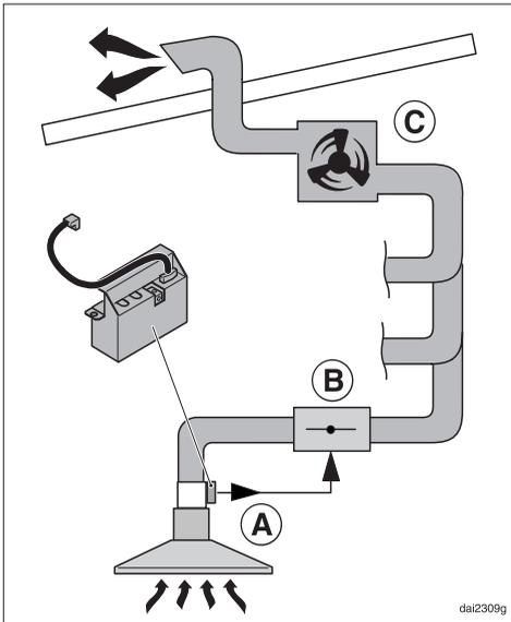
The potential free contact of the DSM 400 ① can be installed in an ...EXT model, for instance, which is connected to a central extraction system.
