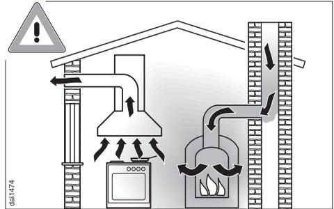
▶ Great care should be taken when using the rangehood at the same time and in the same room or area of the house as another heating appliance which depends on the air in the room. Such appliances include gas, oil, wood or coal-fired boilers and heaters, continuous flow or other water heaters, gas cooktops or ovens which draw air in from the room and duct exhaust gases out through a chimney or extraction ducting.
