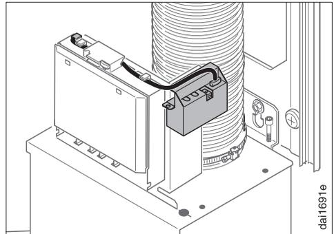
The tower needs to be removed before the control module can be fitted to the fan unit.
