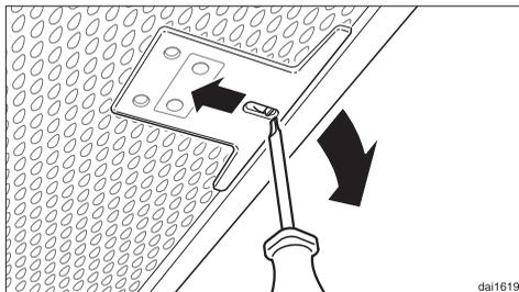
If the grease filters are inadvertently replaced upside down, insert a small screwdriver blade into the slits to disengage the clip.
