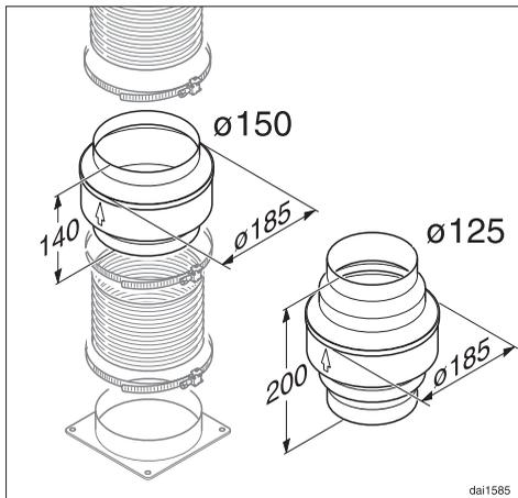
For installations in areas where the exhaust ducting is exposed to cold temperatures, we recommend insulating the exhaust ducting and installing a condensate trap to collect and evaporate any condensate which may occur. Condensate traps are available for Ø 125 mm or Ø 150 mm ducting.
