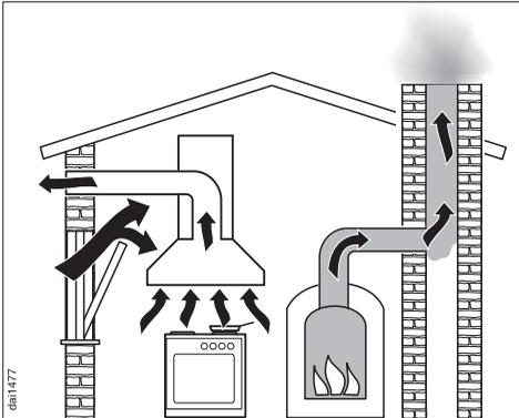
Ventilation can be maintained by air inlets which cannot be blocked, in windows, doors and outside wall vents, or by other technical measures, such as ensuring that the extractor can only be switched on when the heating appliance is switched off or vice versa. A ventilation brick alone is not generally sufficient to ensure safe ventilation.
