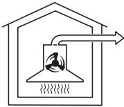
The air is drawn in and cleaned by the grease filters and directed outside.
