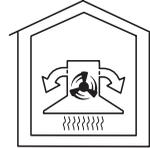
The air is drawn in and cleaned first by the grease filter and then by a **charcoal filter**. The cleaned air is then recirculated back into the kitchen through grilles in the top of the rangehood extension piece.
