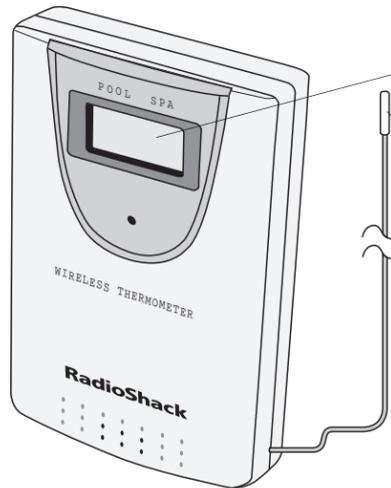
**Liquid Crystal Display** — The current temperature and selected channel appear.
