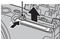
To remove the memory card, press it in and release it slowly. The card can then be removed by hand. When a memory card is removed, the card could come out of the slot too quickly. Use your finger to hold it and gently release the card.
