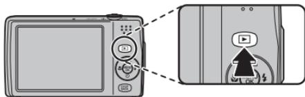
Press the **▶** button again or press the **ON/OFF** button to turn the camera off.
