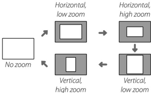
The frame is displayed as shown at right. The composition can be adjusted using the zoom control.
