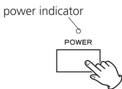
If the power indicator is red, press the ON button of the remote control unit to turn the unit on (see page 11).
