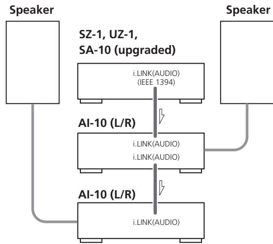
The MASTR and SLAVE settings of the iLINK remote control function allow you to set one AI-10 as master and the other as slave, so that the volume, muting and dimmer of the two AI-10's can be controlled in unison using one of the pair units.
