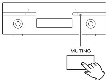
To mute the sound temporarily, press the MUTING button. Press the MUTING button again to restore the sound.
