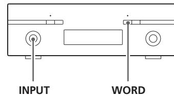
This feature is used when you want to get your whole system locked to a single sync signal (clock) by connecting this unit to the Esoteric SA-10/UZ-1 or other devices that are capable of inputting a sync signal (word clock).
