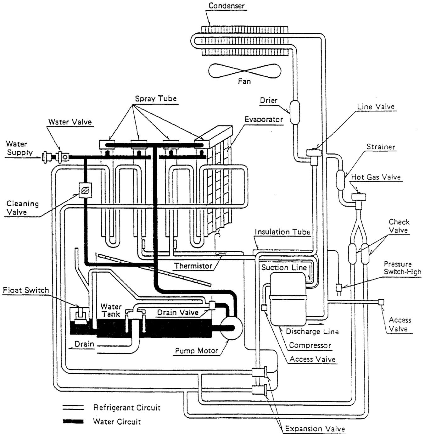
[b] KM-1300MWH (Water-cooled)
