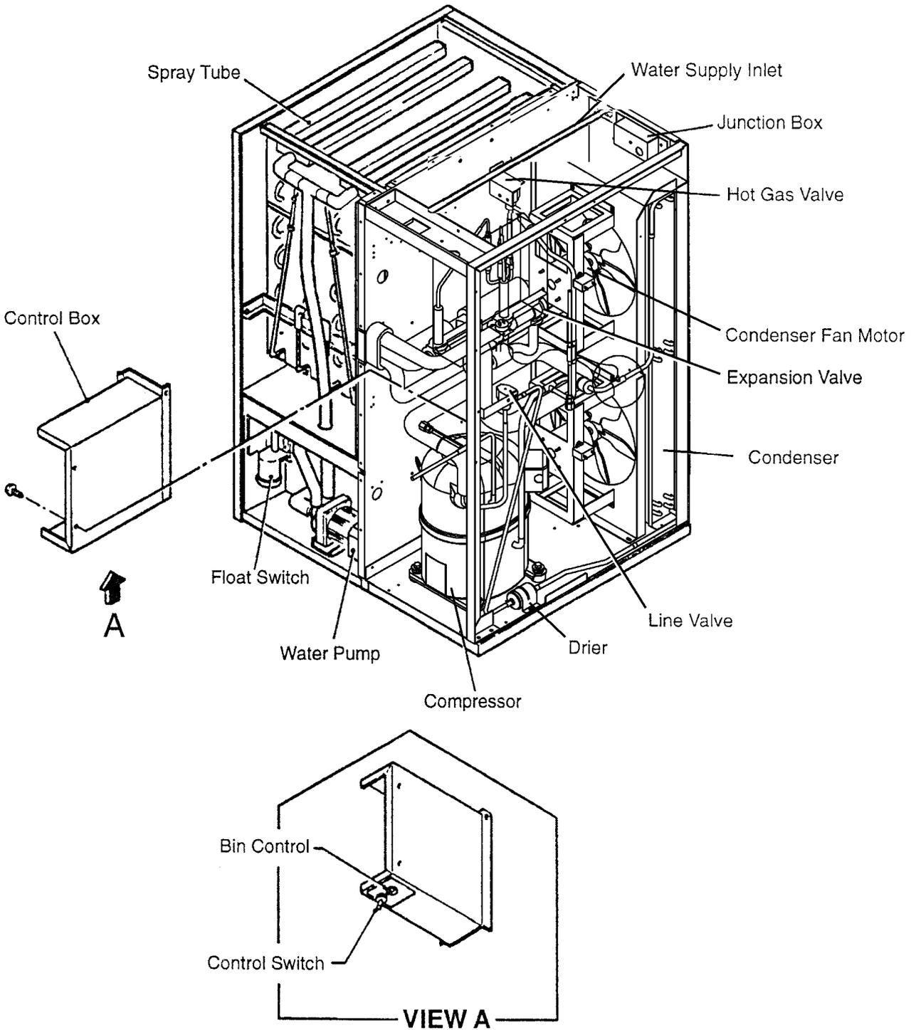
[b] KM-1300MWH (Water-cooled)
