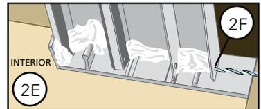
**Note:** Ensure all new or existing weep holes are open before proceeding with the installation.
