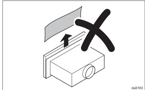
Do not remove the protective film between the deflector plate and the casing until the hood has been placed in the housing unit.
