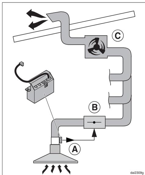
The potential free contact on the DSM 400 ① can, for example, be used in a cooker hood with an external motor ...EXT, which is connected to a central ducting system.
