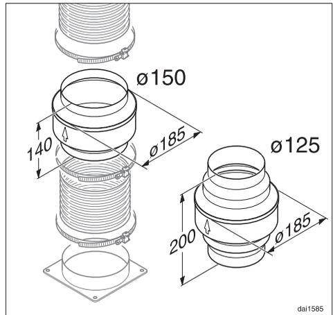
In addition to insulating the exhaust ducting, we recommend that a suitable condensate trap is also installed to collect and evaporate any condensate which may occur. Condensate traps are available for Ø 125 mm or Ø 150 mm ducting.
