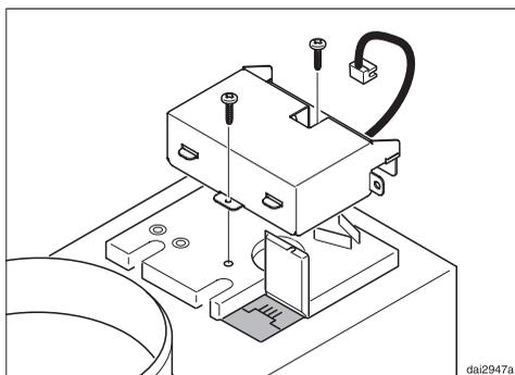
The control module must be installed above the cooker hood housing.
