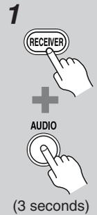
While holding down the [RECEIVER] **REMOTE MODE** button, press and hold down the [AUDIO] button until the Remote indicator lights up (about 3 seconds).
