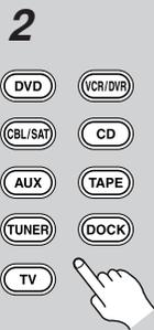
Within 30 seconds, press the **REMOTE MODE** button again. The Remote indicator flashes twice, indicating that the button has been reset. Each of the **REMOTE MODE** buttons is preprogrammed with a remote control code. When a button is reset, its preprogrammed code is restored.
