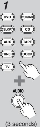
While holding down the **REMOTE MODE** button that you want to reset, press and hold down the [AUDIO] button until the Remote indicator lights up (about 3 seconds).
