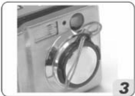
Put the lens strap through the lens strap post.
