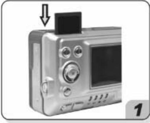
Orient the memory card as shown, and insert it into the slot.
