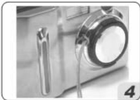
Pull the other end of the strap through the other side of the lens strap post and tighten it.
