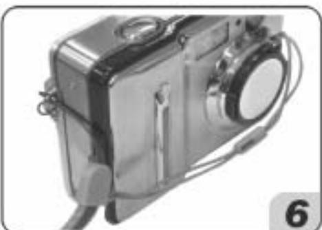
Finally, pull the lens cap through and tighten it.
