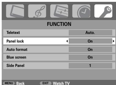
When **Panel lock** is **On**, a reminder will appear when the buttons on the television are pressed. **If the standby button is pressed the television will switch off and can only be brought out of standby by using the remote control.**
