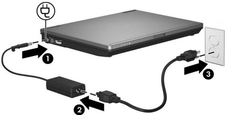
When the computer receives AC power, the battery begins to charge and the battery light (on the front of the computer) is turned on. When the battery is fully charged, the battery light is turned off.
