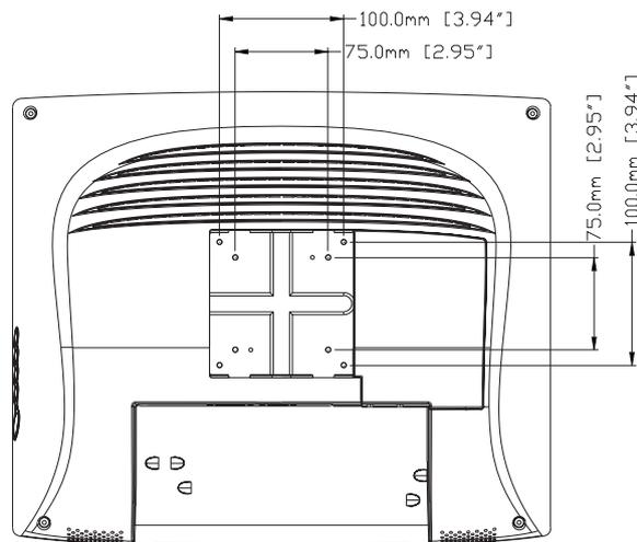
**Note:** The above drawing displays the VESA mounting interface after the removal of the mounting cover and base.
