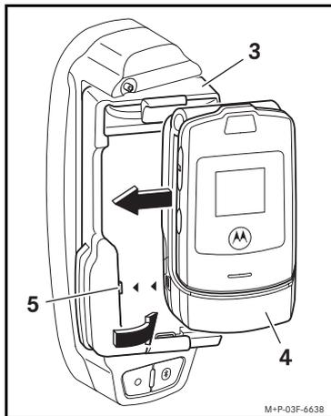
2. Slide the Motorola RAZR phone (4) into place. Make sure that connector (5) connects to Motorola RAZR phone (4).
