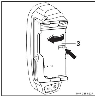
1. Push the latch (3) at the "PUSH"-sign. The latch (3) will swing out.
