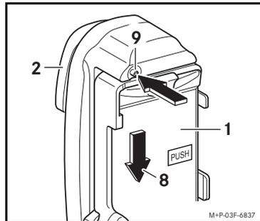
1. Press and hold the release button (9). Slide the Mercedes-Benz V3 Cradle (1) in direction of arrow (8) and remove it from the pre-installed contact plate (2).
