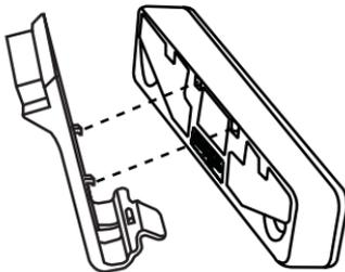
2. Push the Sound Bar down and back into the Sound Bar Bracket.
