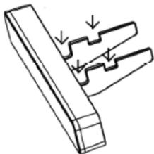
3. The viewing angle of the device in the stand can be adjusted by moving the two stands as shown.
