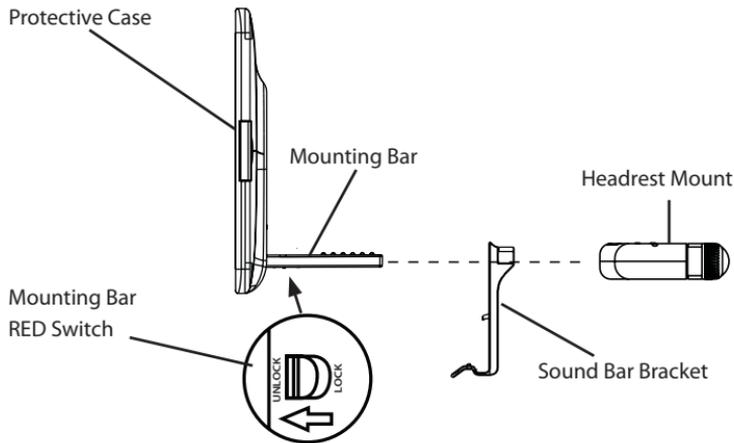
1. Hold the **RED** switch on the Protective Case in the **UNLOCK** position.
