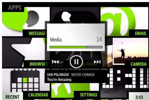
While in the Music & More app, press one of the VOLUME buttons to open the media controls overlay. The controls will auto-dismiss after a few seconds, but you can always dismiss them manually by pressing the BACK button.
