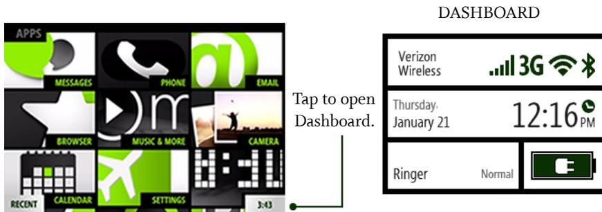
The mini Dashboard always displays the most relevant status information, depending on what you're doing. For example, if you're on a call, the mini Dashboard indicates whether you're roaming and your signal strength.
