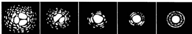
Figure 5-1. Seeing conditions directly affect quality. These drawings represent a point source (i.e., star) under bad seeing conditions (right). Most often, seeing conditions produce images that lie some where between these two extremes.
