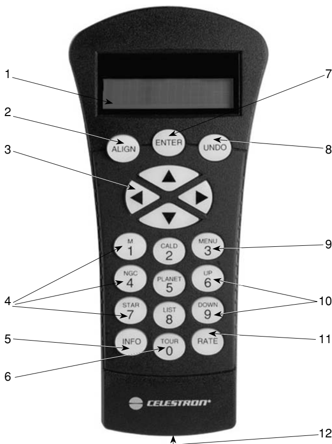
Figure 3-2. The StarSeeker hand control
