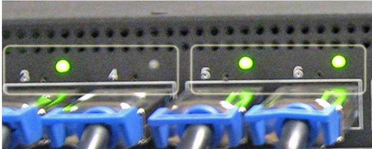
**Note:** Ports 3 and 4 illustrate a x8 connection with a single LED lit while Ports 5 and 6 illustrate two independent x4 connections with a LED lit for each port.
