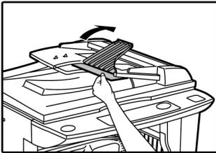
**2** Open and close the ADF to make the misfeed location indicator stop blinking.
