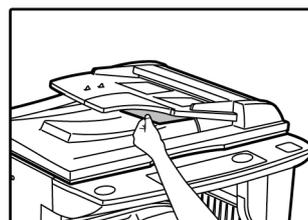
If a small original (A5 (ST), etc.) is misfed, open the right side cover and remove the original. Close the right side cover.
