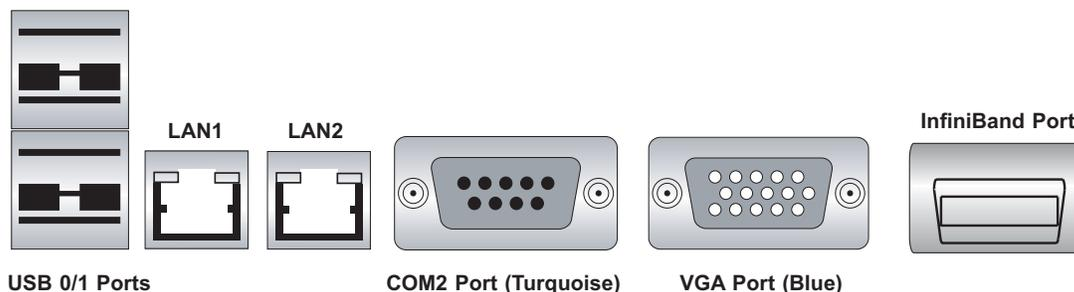
**Note:** InfiniBand ports are included on the X7DBT (6015T-INF) only. To prevent damage to the port or serverboard, an InfiniBand bracket (included) must be used to secure the connector to the I/O shield.
