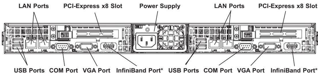
\*The InfiniBand ports are included on the 6015T-INF only.
