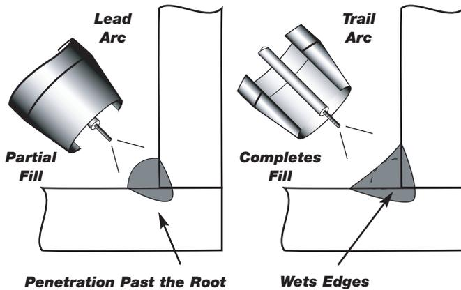
*The Lead Arc generates the majority of the penetration and leaves joint requiring additional fill.*
