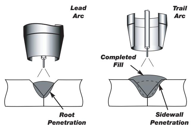
*The Lead Arc creates the initial root penetration and the majority of the joint fill.*
